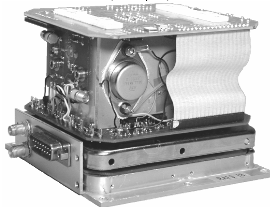
Fig 2: Picture of RAFS1 without external cover (before update)
